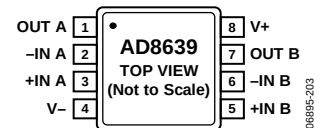
Figure 3. 8-Lead MSOP (RM-8) 8-Lead SOIC_N (R-8)
